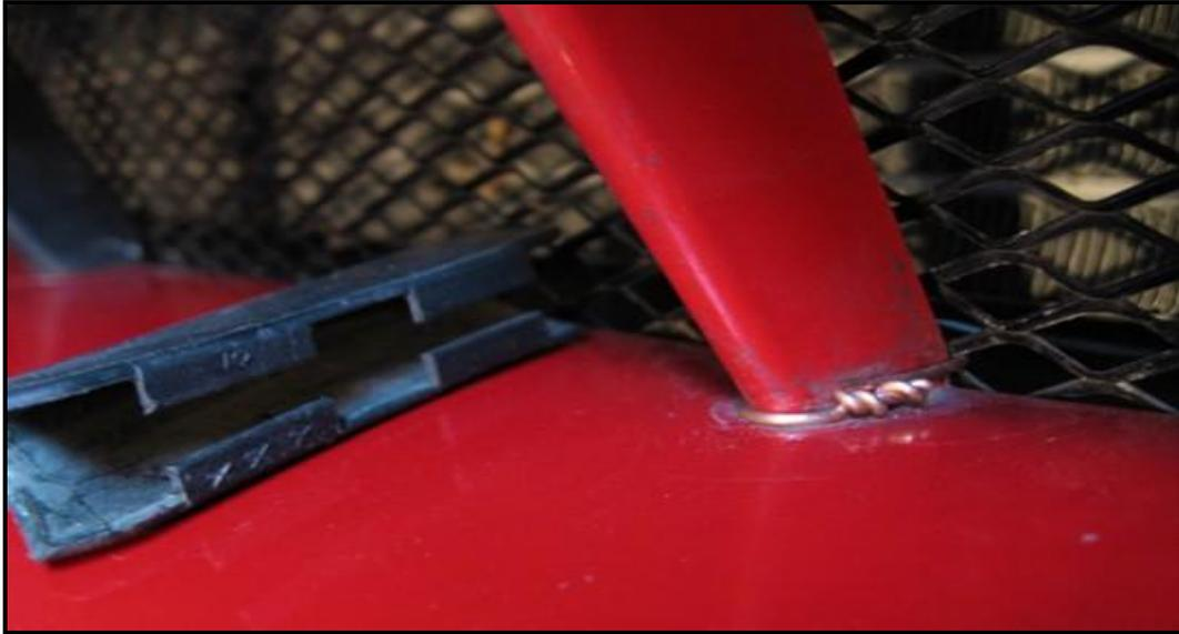
On the sw20 grille there are two groups of five vertical bars which have a fixed core covered by a trim that fits over the top. Remove the trim pieces from the *lower five bars* by reaching in and spreading the rear, which will allow you to take them off.
