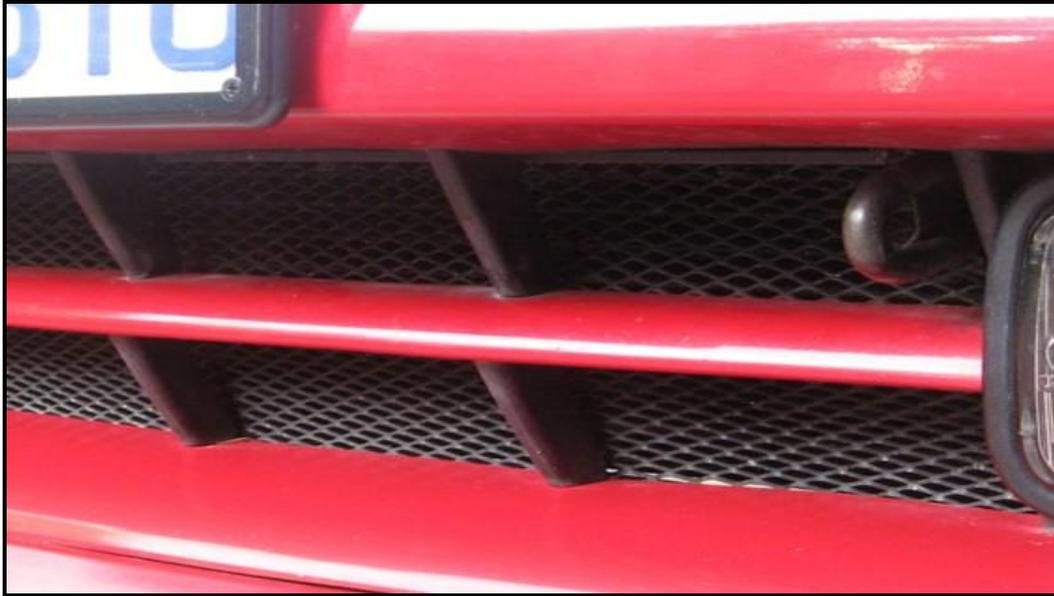
After having to fit a new airconditioner condenser core due to impact damage I was looking to find a way to protect it, and I discovered that it was relatively easy to fit a protective mesh in front of the core, sliding it in diagonally from the top.
