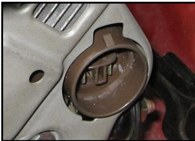
You will need to disconnect the wires from the alternator. Fold back the rubber boot, undo the nut and remove the main alternator wire.
