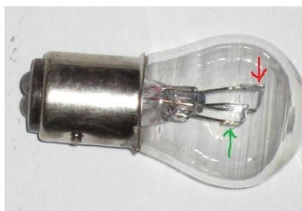
9. Note the colour wire on the new socket which controlled the tail filament. It's safe to assume that the other wire will control the brake filament, but if you want to be sure connect it to the other side of the loom (using the green w/white stripe wire) and repeat the process, although you will need an assistant or a heavy weight to keep the brake pedal held.
