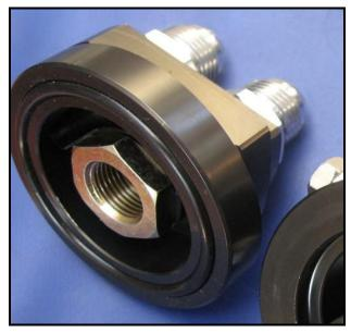
Care was needed when fitting the hoses between the engine adaptor and filter mount. They go: outside connector to outside connector (pre filter), and middle connector to middle connector (post filter).
