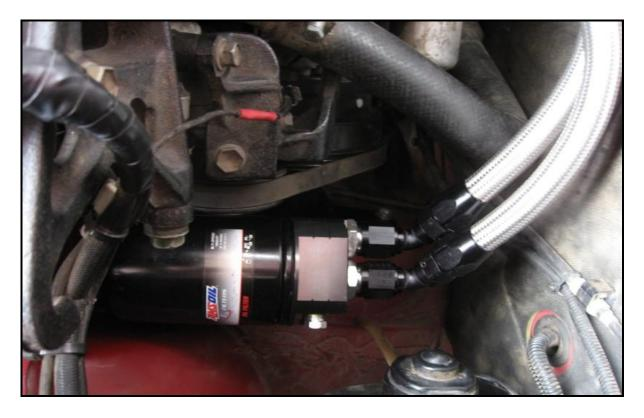
I found 2 unused holes (turbo intercooler mounts) already tapped into the chassis rail conveniently just below where I wanted to mount the filter, so I used them to hold the mounting bracket.
