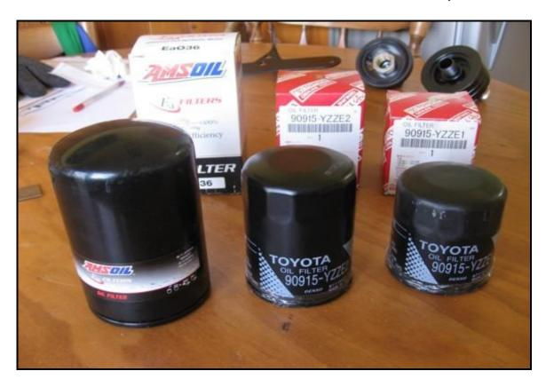
Of the 3 filters shown, the 2 smaller ones will both fit both NA and turbos in the OEM position, and you can easily see how much larger my new filter is compared to the other 2.
