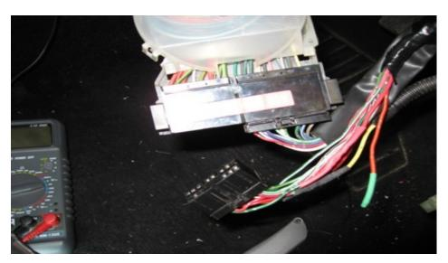
The 12 volts to power the relay coils I got from patching into the W-R wire, (post h/lamp relay and pre h/lamp fuses) underneath the fuse box.
