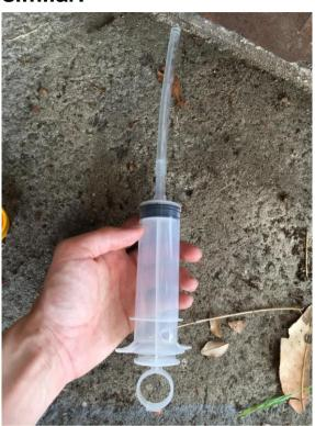
4. Fill the syringe about ¾ full of brake fluid and ensure that no air is left in the top of the syringe or tube that's attached otherwise you'll pump air through which is what we're trying to avoid.
