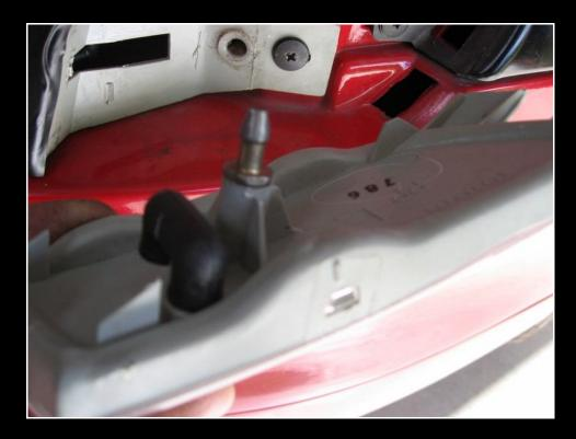
To get it out, one thing that really helps is to use two flat bladed screwdrivers to lever the side reflector out. (Similar to the way tyre levers were used to remove a tyre from the rim).
