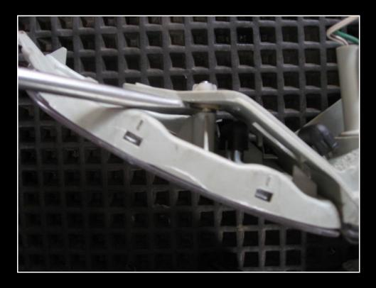
After you replace the globe and the parker/lens assembly, to refit the side reflector simply push it in until it clicks into place, but first it might be a good idea to smear a bit of grease on the lug to help get it off the next time you want to change a globe.
