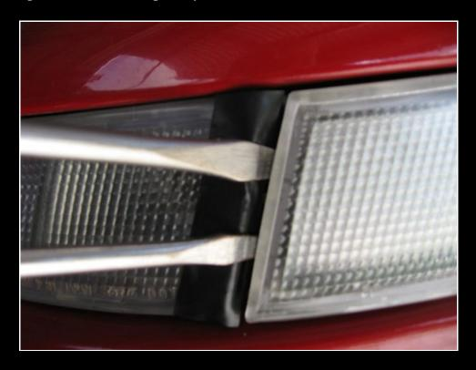
Once the side reflector is off you can easily remove the screw and take out the parker assembly. To change a globe, simply twist the globe holder to get it out.
