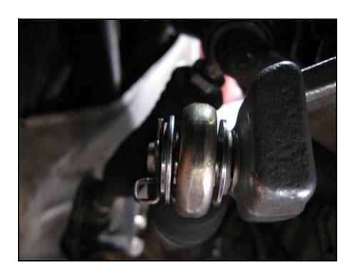
When both cable ends are fitted, and their holding clips inserted, you only need to refit the air scoop and lower the car. Job finished.
