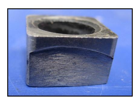
The picture shows the wear I found on the block (about ½ mm each side) that doesn't seem like much. But it all adds up, because as I've mentioned before, this slack is magnified at the gear knob.
