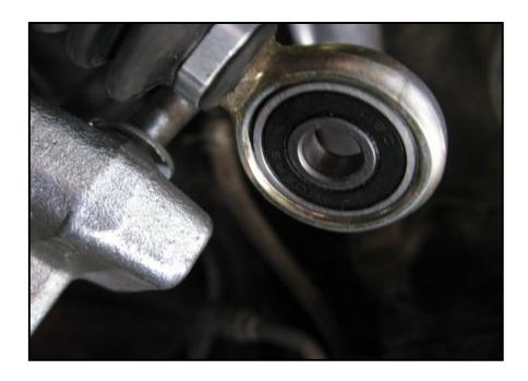
Below is an end view, showing the washers. I used six altogether on each cable, but this could vary depending on the thickness of the washers you use.
