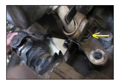
The block was only worn on 2 sides so I simply rotated it 90 degrees, greased it and put it back, but on some cars the block may have already been rotated so it might be a good idea to get a new one from Toyota before tackling the job just in case.
